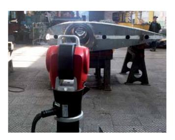
The Center conducted dimensional check of shipbuilding units, such as:
